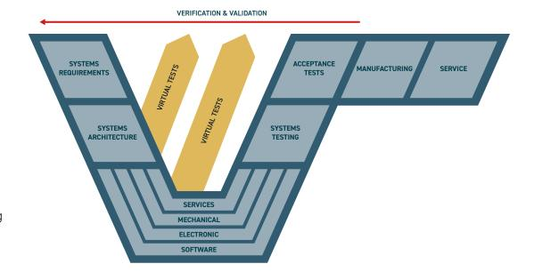
The V-Model is the classic graphical representation of the systems development lifecycle—from requirements, to cross-discipline design, to testing, and verification and validation. The left side of the "V" represents the creation of requirements and system specifications. The right side of the "V" represents integration of parts and their validation. Organizations must use the V-Model as the anchor for communication and design work in complex products.
